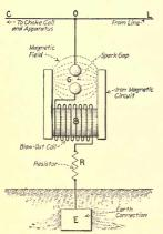
Fig. 153.—Illustrating the principle of the magnetic blow-out lightning protector.
